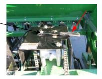
Remove the black box on the left side of the drill to access the location where the sprockets can be
