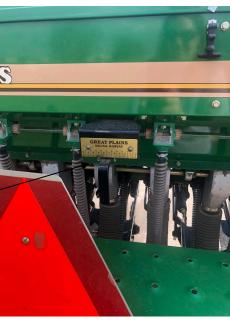
See page 38 of the operator's manual for information on setting press wheels for seed depth. T handles should be closer to implement for shallower seeding and further away from implement for deeper seeding. Each increment adjusts depth by approx. 1/8th of an inch. Depth range is from 0 to 3 ½ inches
